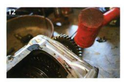
engage any two shift forks with any two gears simultaneously. Then, with the mainshaft effectively locked, take a thin-head gear wrench and loosen the nut by turning "backward," ie. clockwise (photo 7). When it's loose, move the forks back and disengage the gears. Take out the side-cover bolts and the whole assembly will pop off, leaving the shift forks and two shift cams sticking out of the cover.
